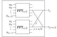
We're using a particular shorthand: the edges are wires carrying complex numbers from left to right. A weight of j means "multiply the number on this wire by  $\omega^j$ ." And when two wires come into a junction from the left, the numbers they are carrying get added up. So the two outputs depicted are executing the commands
