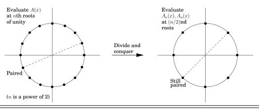
Figure 2.7 The fast Fourier transform (polynomial formulation)
