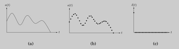
In order to extract information from a signal, we need to first *digitize* it by sampling (Figure (b))—and, then, to put it through a *system* that will transform it in some way. The output is called the *response* of the system:
